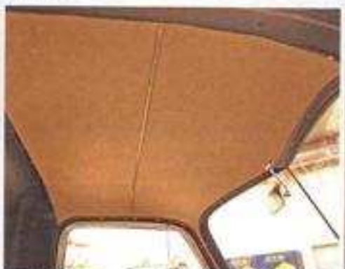
The headliner insert is held in place with the stock moldings, and a polished bow adds a touch of class.
