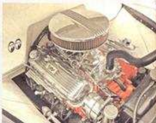
The nicely detailed big-block Chevy engine displaces 468 ci and pumps out 375 hp. A Demon carburetor tops the polished intake.
