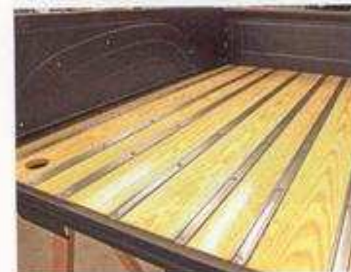
The new wood in the bed is accented by the brushed-finish stainless steel strips.
