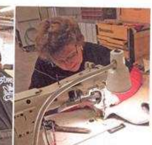
The seat covers are being stitched. The seat is a custom-made piece, and the rolled and pleated leather will go a long way in terms of style and comfort.
