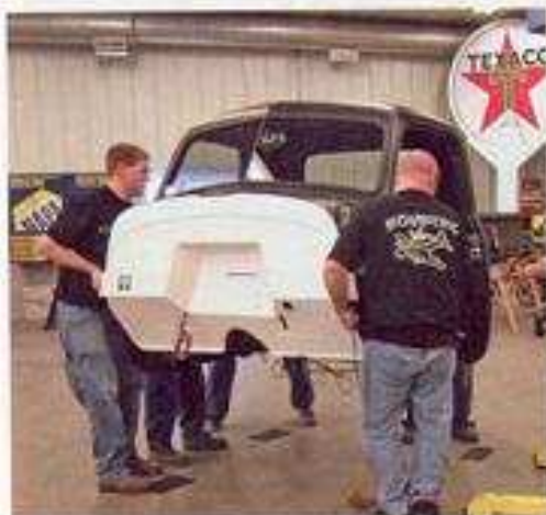
A little grunt work is done in order to get the cab up on the cherry picker-turned-body boom.
