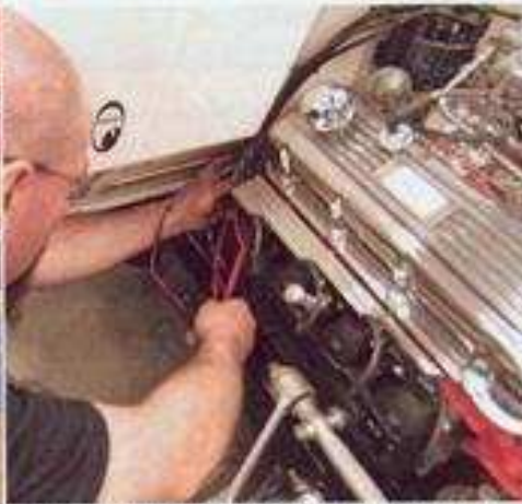
Wires to the starter and alternator are neatly routed forward. A Centech system was used in the truck.
