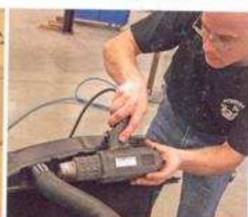
Large shrink wrap covers the hose clamps, and a heat gun does the shrinking... details, details, details.
