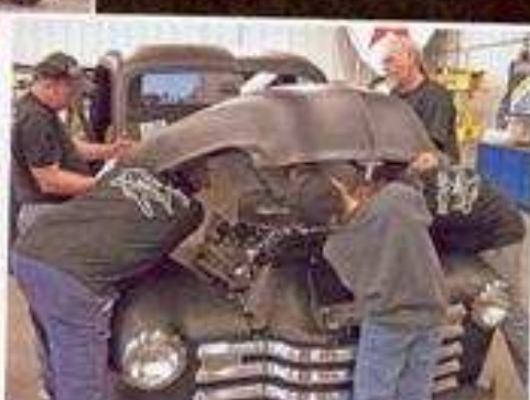
The next piece of sheetmetal to go on the truck was the hood, and since most of the work was done at this point, there was no shortage of helping hands!
