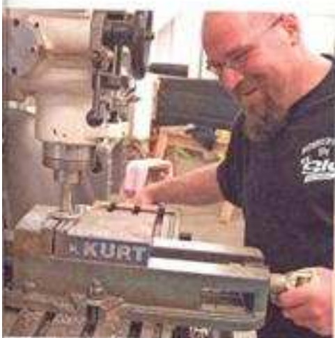
When the floor escutcheon for the steering column didn't fit, it was time to mill a little clearance.
