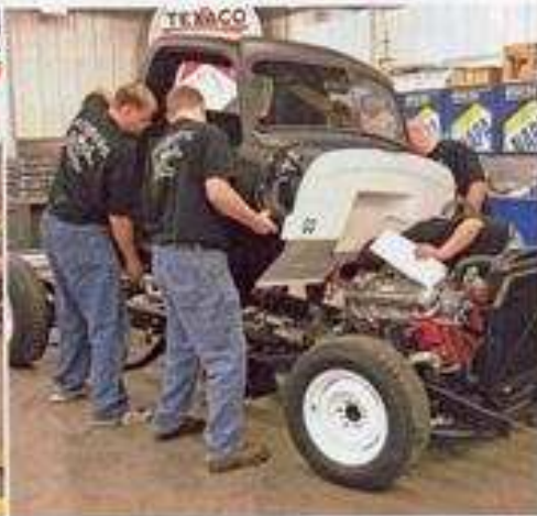
The cab is slowly rolled into place as the bomber crew steadies the cab.
