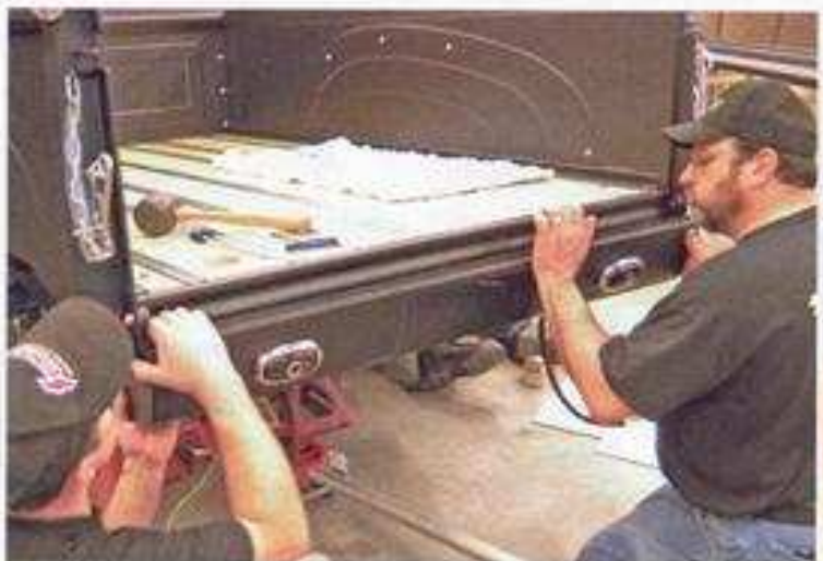
The custom-built rear pan and '47 Chevrolet taillights are bolted in place.
