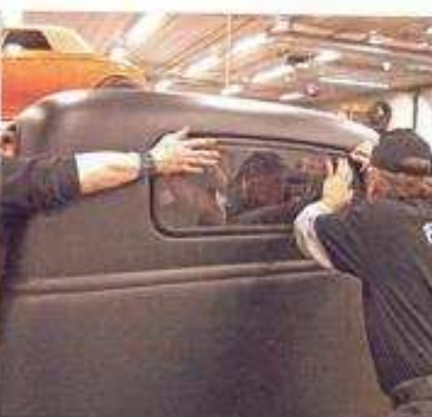
A tinted rear window and new rubber are pressed into the cab.
