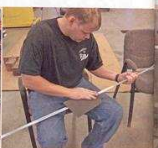
Before the stainless steel bed strips were installed, they were brush-finished with a piece of Scotch-Brite.
