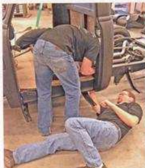
Body bolts come next. One guy in the cab and one guy under the cab makes it quick and easy.
