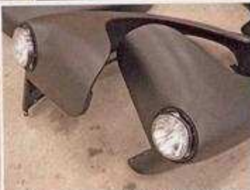
Headlights are mounted in the front fenders, and they're ready to be fit to the truck.
